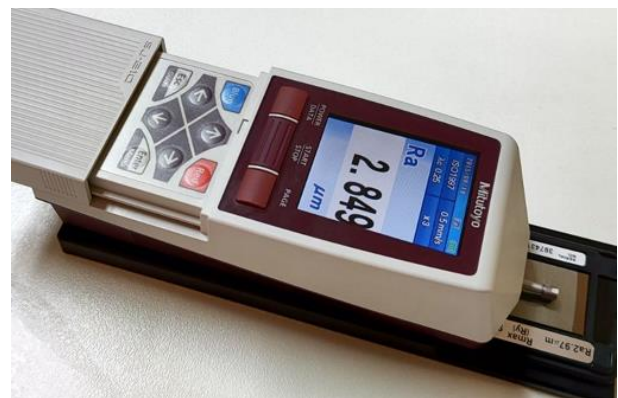
Fig. 4 Mitutoyo SJ 210 roughness tester.
