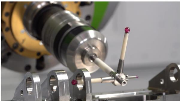
Fig. 3 Measurement Directly On CNC Machine [2].
