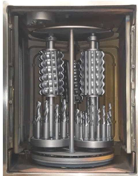
Fig. 6 Mixed batch: the upper level performs 2-axis and the lower - 3-axis rotation in equipment π80+ (Platit AG).
