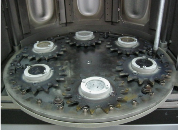
Fig. 1 Cycloidal lantern gearing of a carousel designed for use in equipment HVP100RHD (Milko Angelov Consulting Co.).
