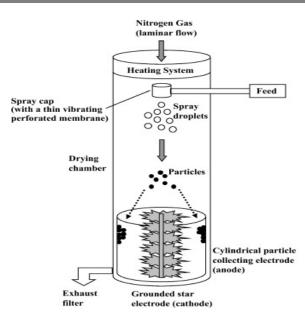
Fig. 3 Mechanism of nanoparticle formation using nano spray drying technique.
