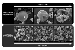
**Fig. 5** Effect of the production parameters to the morphology.
