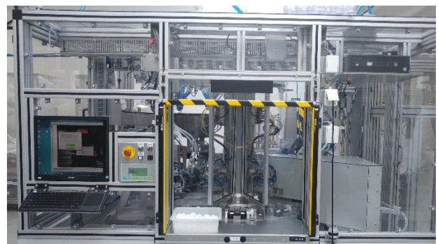
Fig.1 Station for automatic inspection of final product after assembly.
