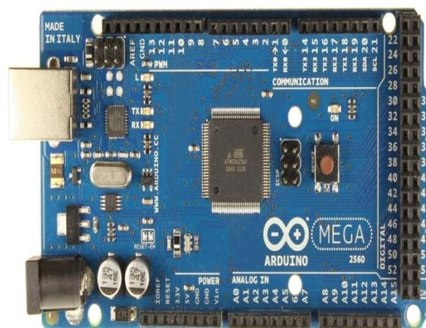
**Fig. 1** Appearance of ARDUINO MEGA 2560 board
